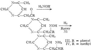
The 4-acetonyl- and 4-phenacyl-2,6-dimethylpyrimidine were converted to the corresponding oximes by treating them with hydroxylamine hydrochloride in a pyridine–ethanol solution similarly to the procedure of Bachmann and Boatner.<sup>9</sup> These ox-
